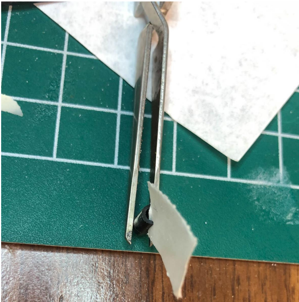
Figure 1. A thin piece of styrene is in the radial break in the Bowser axle sleeve. Replace the sleeve and problem solved!
