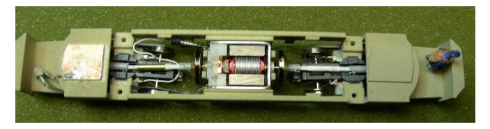
The frame with the Halling drive installed. The plugs on the ground wires from the trucks can be seen at the upper left of the motor. The plus wire goes from the motor to the plate at the left where a spring wire from the pole base makes contact with it. Note the miniature plug on this wire next to the plate. All these plugs allow the motor and trucks to be removed without un-soldering.
