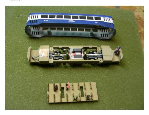
The above photo shows the three components, body, frame, and seat/floor. Besides providing seats, the floor anchors the drive in place.
