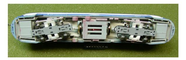
The underside has weights below the platforms. There are also weights above the platforms in the ceiling.
