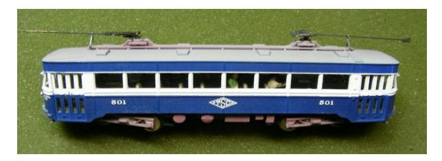
The finished car has not plied the streets of Scranton for very long as the culm on the roof and underbody is not very heavy. The triangular pole hooks fit under the trolley boards – they were hard to glue in place but they will stay there.
