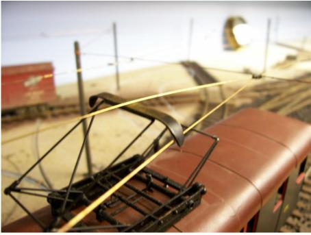
How to make hangers that place running wire enough below span wire to prevent Pan snag on span.
