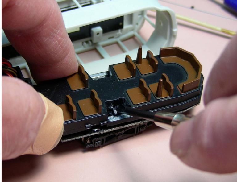
I removed some of the floor by first filing away a little of the edge that stops the truck tabs. Just file up through the holes at the end of the curve of the hole. Caution – be sure the motor is protected from filings or the car will grind to a halt on the first test run. See the photo below.
