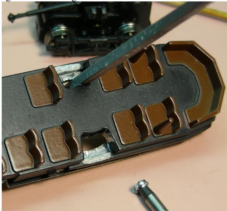
Once all eight edges are filed use a Dremel motor tool with a cutting bit as shown in the photo below (the same bit as appears above). Get this bit down on the lower flat curved surface and cut
