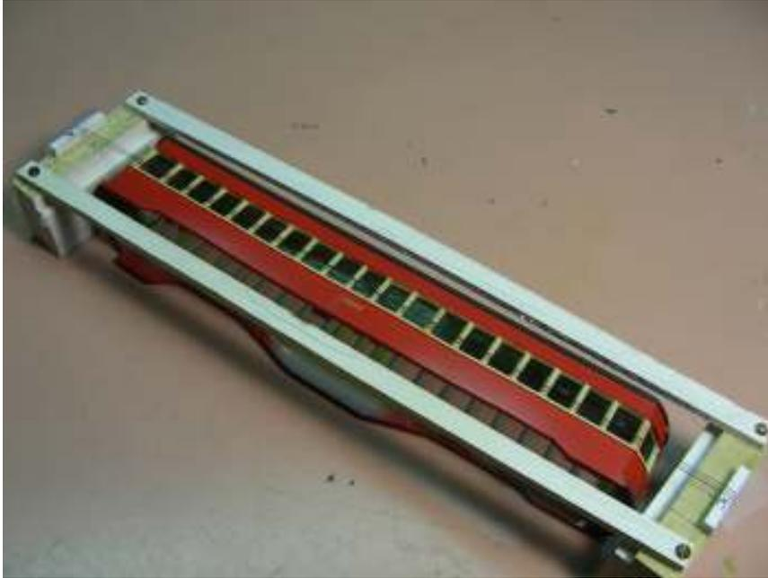
Lay the loom over the car – the car should be slightly higher than the EZ Line so it stretches it just a little more. Get the EZ Line aligned to its proper position.
