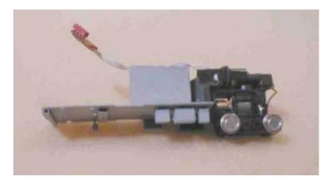
The underbody assembly is shown here. The blocks behind the motors and in the two center cars are weights, necessary to make the hills on Bob's layout. Because of those grades the whole train is assembled with excess play in the drawbar screws.
