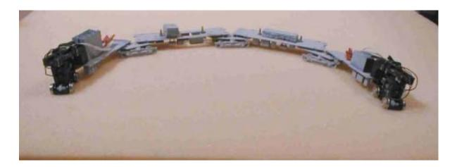
The modified liner can bend around a 6" curve, something the prototype was never asked to do. The finished product heads into a curve on Bob's home layout.
