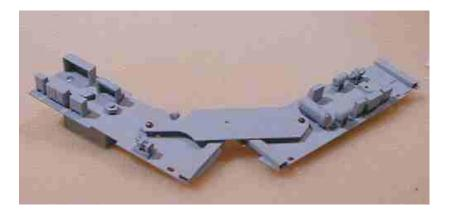
The Bachmann frame is cut in half, the fuel tanks removed, and drilled and tapped for 2-56 screws. The floors of the Liner end units are cut back to match and attached to the Bachmann frames.
