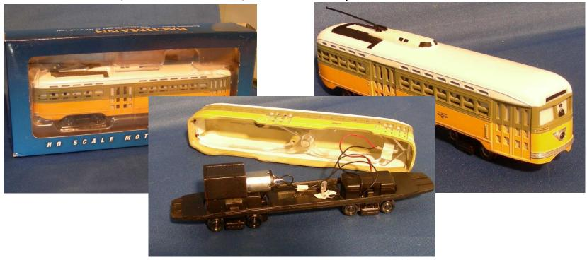
Bachmann recently, & quietly, released a new drive for their PCC It has a truck-mounted can motor and enclosed gear box. Similar quality as the Peter Witt.
