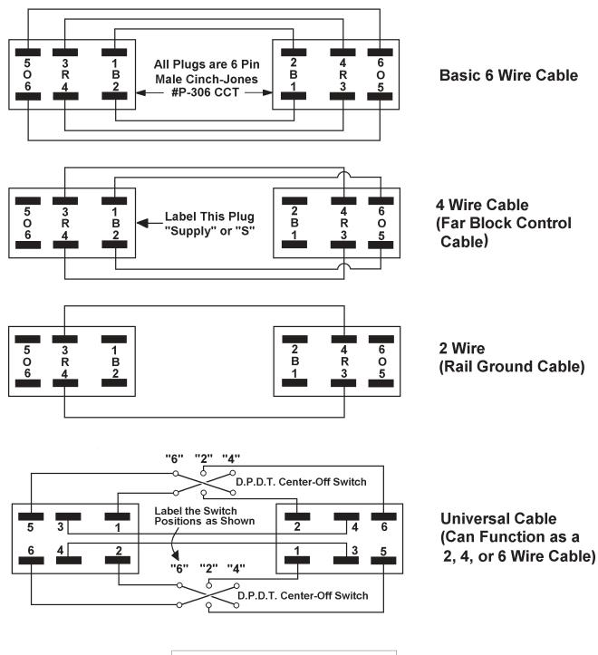
Pins 5 & 6 - <u>O</u>verhead Wire Pins 3 & 4 - <u>R</u>ails Pins 1 & 2 - <u>B</u>lock Control
