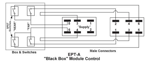
To use the Black Box, plug the supply-side connector (it has four wires) into the socket on the module you will be controlling from. Plug the other connector (with six wires) into the adjoining "controlled" module. Finally, clamp the Black Box to the module edge with a small C-clamp.
