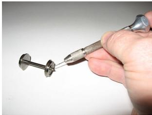
2. Start drilling at an angle towards the axle, until the bit starts into the insulating material. Then carefully straighten the drill, parallel with the axle, and drill through to a depth equal to the thickness of the wheel. You will hit a “shoulder” on the axle inside of the wheel, or see the drill bit come through on the inside of the wheel. The drilling should be easy, through plastic or nylon. Buy several bits – the tips can break!
