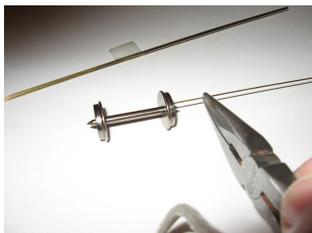
3. Use needle-nose pliers to carefully insert the brass wire the full depth of the wheel thickness. Then bend the wire up and away from the axle end at about a 45-degree angle. This makes it easier to snip off close to the bend. I use Xuron flush-cut rail nippers. Leave enough wire so that you can bend it all the way over, flush to the wheel, and can grab it later (see below).
