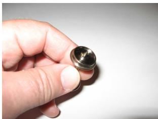
4. Use needle-nose pliers to bend the wire piece the rest of the way, squeezing it flat against the wheel's hub. I then use a screwdriver tip to rotate the wire slightly, so that the exposed portion lays flat on the axle, instead of pointing away from it. This hides it better behind the truck's journal box. Test the electrical continuity between the axle and the wheel with an ohmmeter. The reading does not have to be zero ohms, just a low number. Do the other wheelsets, then carefully twist
