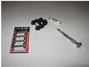
1. To remove and replace wheels from the truck, twist the sideframes and carefully extract or insert the wheelsets without damaging the axle point or the surface it revolves in. Do it carefully and the truck springs will not pop out. (An Athearn O-scale archbar truck is shown. Its plastic wheels will be replaced with metal Intermountain wheelsets. With Atlas O trucks, you must unscrew the sideframes and bolsters.)
