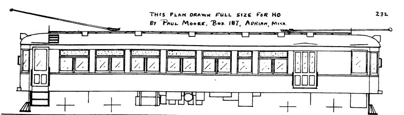
BRILL MCB-27 TRUCKS - 7' WHEELBASE -36" WHEELS - 4 - 160 H.P. MOTORS - MCB RADIAL COUPLERS
